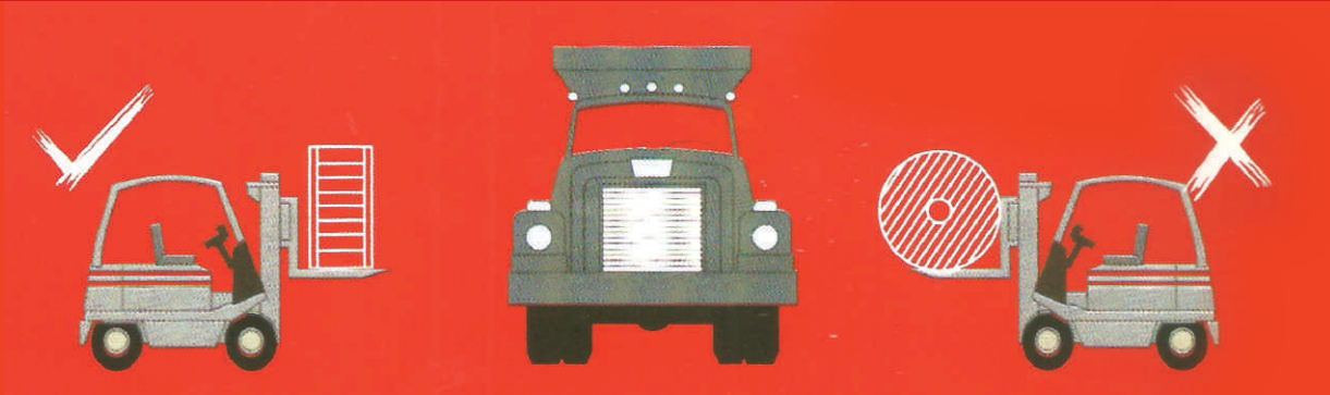
Lift Drums on Fork Trucks
